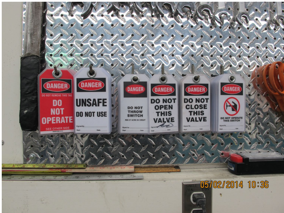
Figure 21: Lockout-Tagout Station in the Machine Shop
